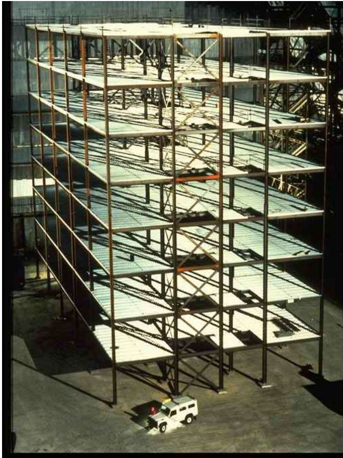
Fire Safety Engineering: test di incendio, Cardington (1998)
